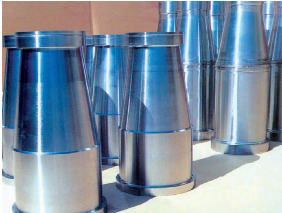
Separating Technology: Decanter Shells weld assembly from horizontal and vertical centrifugal castings
